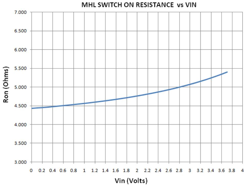
Figure 15. ON-Resistance vs. VI for MHL Switch
