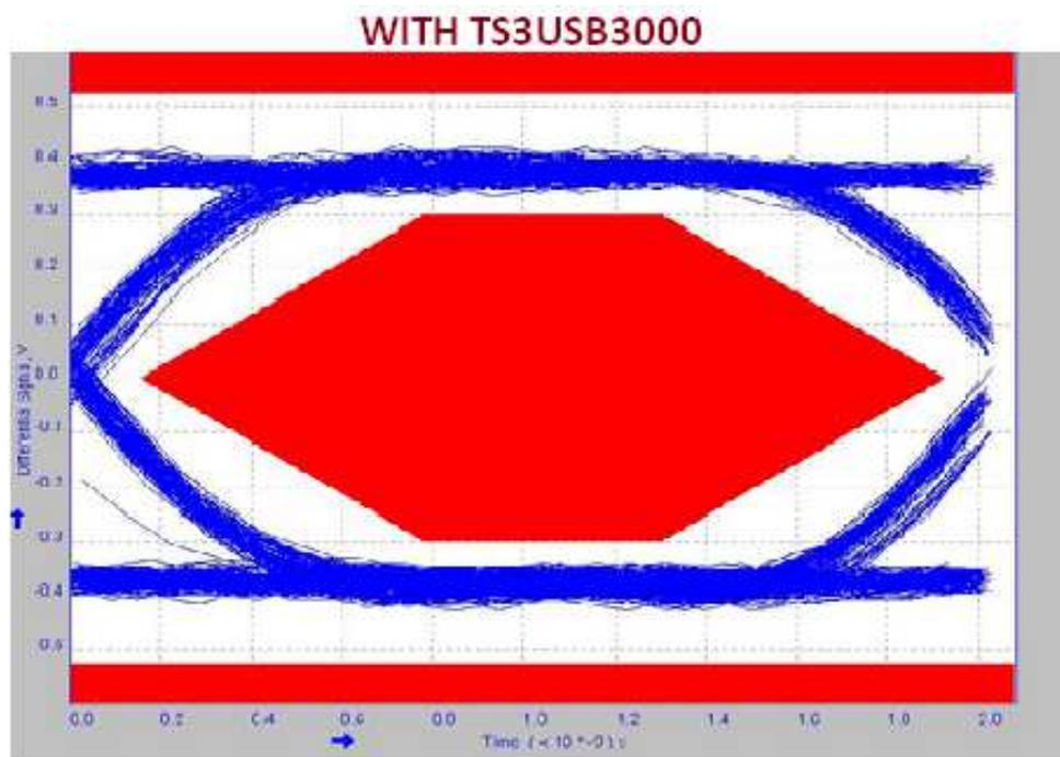
Figure 14. 480-Mbps USB 2.0 Eye Pattern for USB Switch
