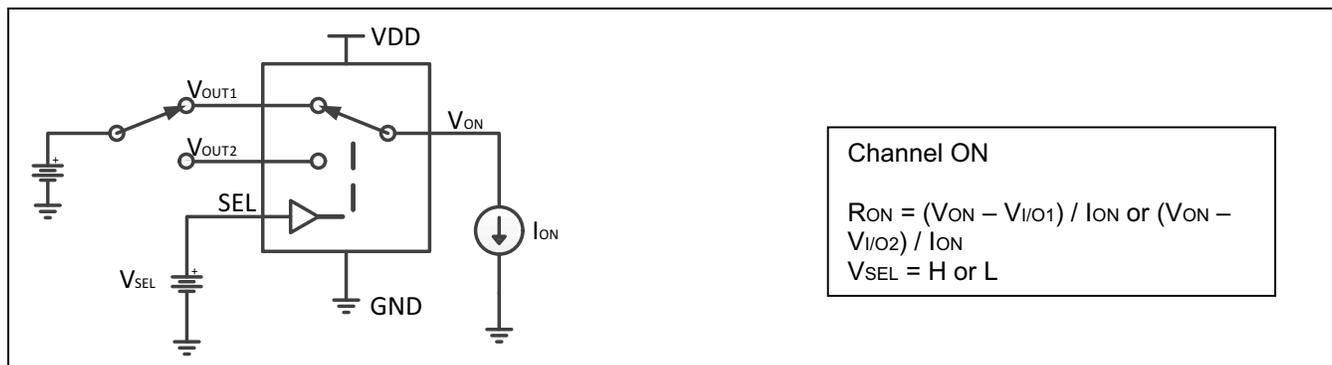
Figure 2. ON State Resistance ( $R_{ON}$ )
