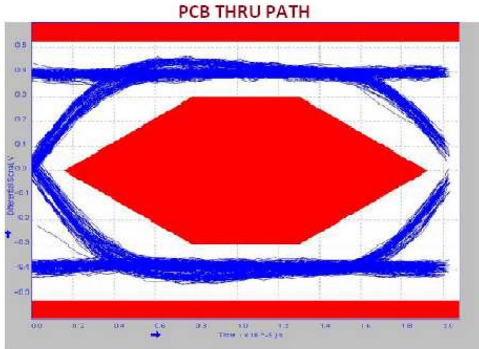
Figure 13. 480-Mbps USB 2.0 Eye Pattern with No Device
