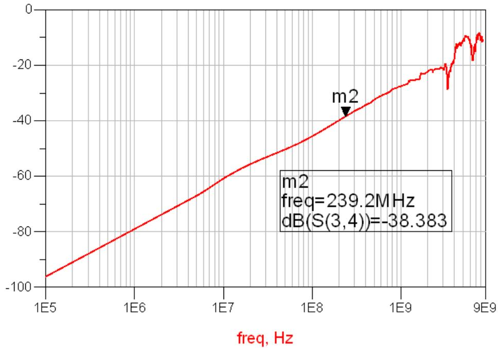
Figure 21. Cross talk vs. Frequency for MHL Path
