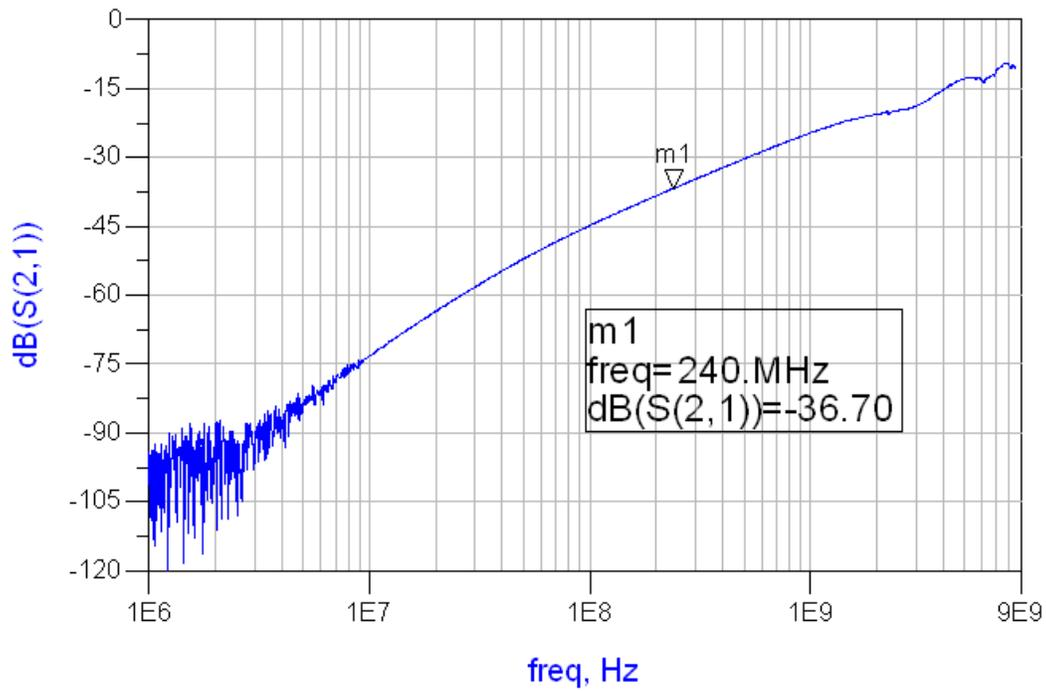
Figure 19. Off Isolation vs. Frequency for MHL Path
