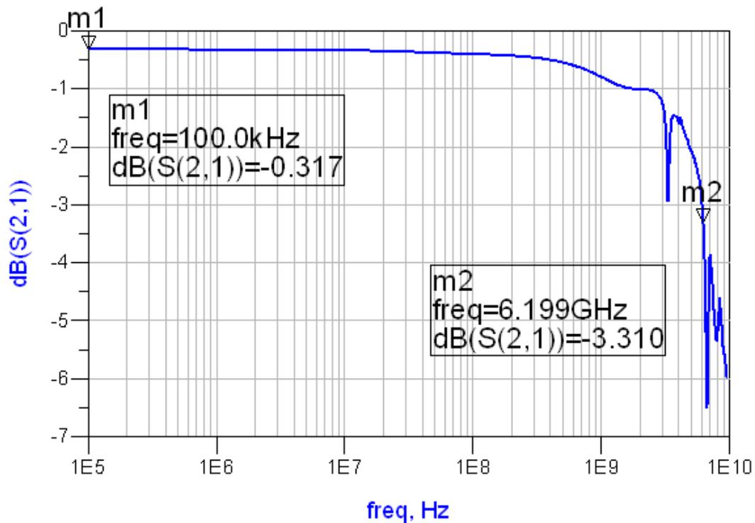
Figure 18. Differential S21 vs. Frequency for USB Switch
