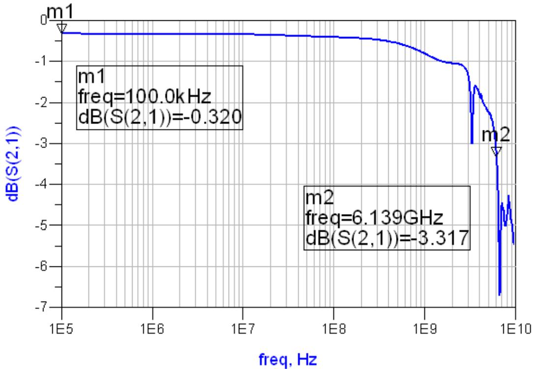
Figure 17. Differential S21 vs. Frequency for MHL Switch
