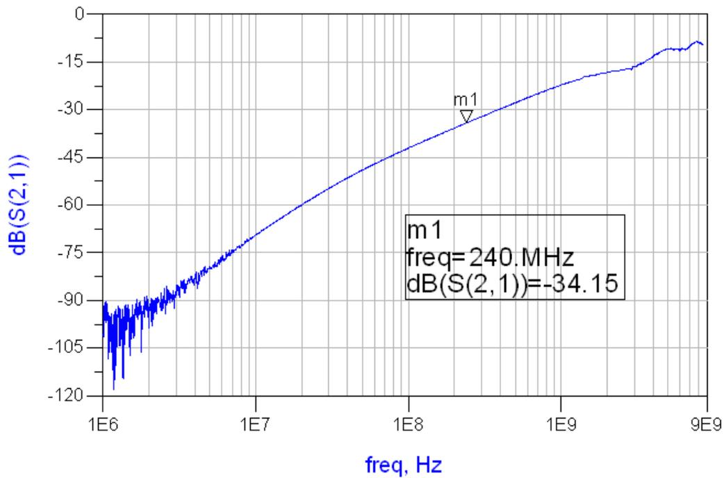
Figure 20. Off Isolation vs. Frequency for USB Path
